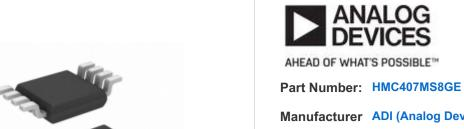
Manufacturer ADI (Analog Devices, Inc.) **Description** IC RF AMP GP 5GHZ-7GHZ 8SMD
